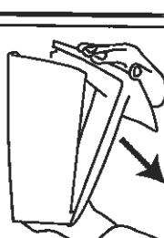
1. Open the dispenser by pushing up on the release latch. The latch is on the bottom back edge of the dispenser in the center. While pushing the release latch, open the dispenser by placing your other hand on the top and guiding the front cover forward.
