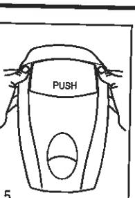
1. Open the dispenser by pushing up on the release latch (or with the key if you have converted to the keyed locking mode). The latch is on the bottom back edge of the dispenser in the center. While pushing the release latch, open the dispenser by placing your other hand on the TOP, and guiding the front cover forward.
