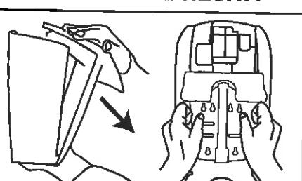
**1. IMPORTANT:** Dispenser opens to the front. For ideal placement, the dispenser should be mounted 3" above any countertop, fixture or obstruction and 2" below any upper cabinet, fixture or obstruction.
