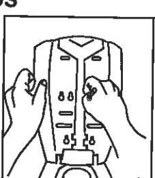
**1. IMPORTANT:** Dispenser opens to the front. For ideal placement, the dispenser should be mounted 3" above any countertop, fixture or obstruction and 2" below any upper cabinet, fixture or obstruction.
